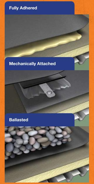
Fully adhered systems are ideal for roofs with unusual or odd-shaped contours, where mechanical penetration of the membrane is not desirable, yet exceptional wind performance is needed. Once positioned over the substrate, the back of the membrane and the substrate are coated with GenFlex bonding adhesive, allowed to dry, carefully rolled back into position and broomed into place.
