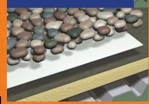
Mechanically attached systems offer exceptional performance in high wind conditions at a very low installed cost. The complete line of fastening accessories assures the right attachment for the right condition.
