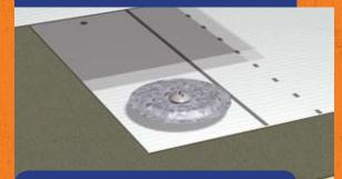
**Mechanically Attached Dual-Weld**
